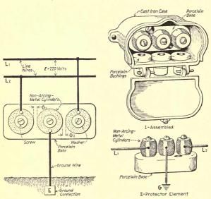
Fig. 160.—Illustrating the principle of the non-arcing metal gap protector.
